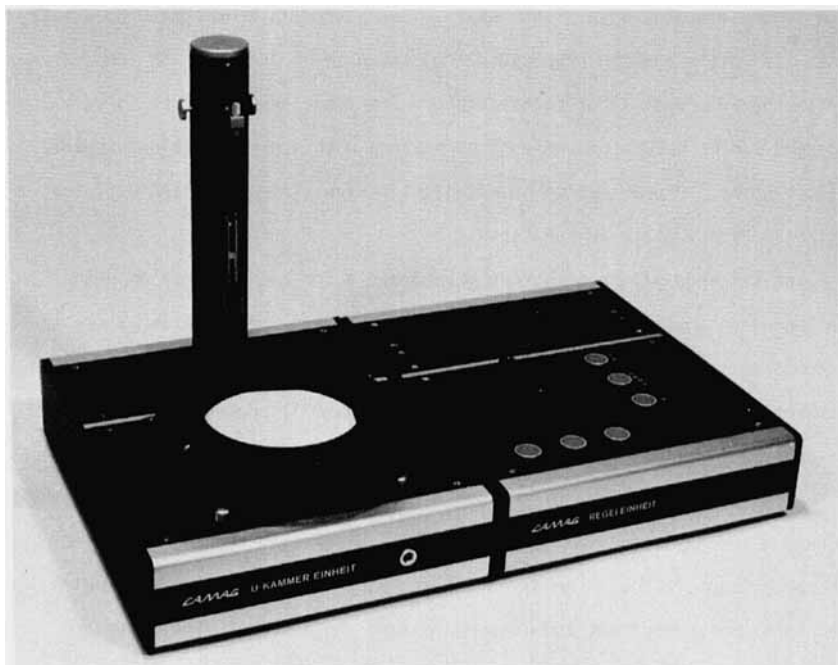
Figure 1: The U-chamber for circular development.
